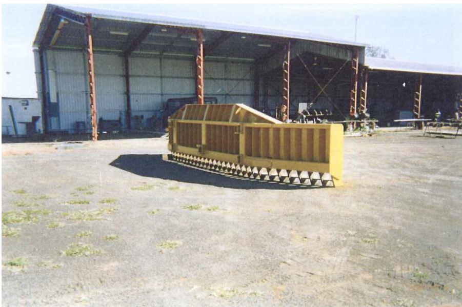
38ft stick rake - Custom made by G. Clarke
