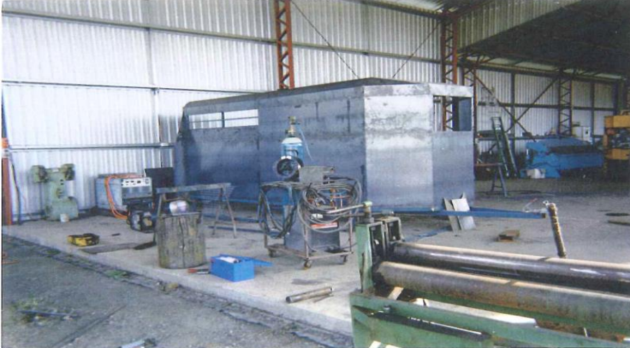
Bull catcher trailer - with electric winch for securing scrub cattle. Custom made G Clarke.
