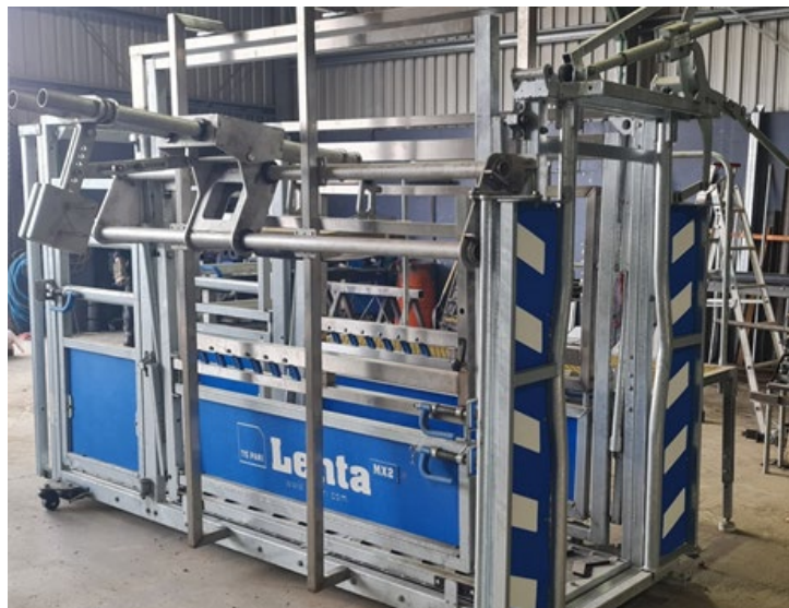
Figure 2 – Initial build of the animal handling unit showing the cantilever assembly for positioning the sensor. Galvanised steel was replaced with stainless steel where necessary. A platform was constructed for the operator to stand on while making measurements.
